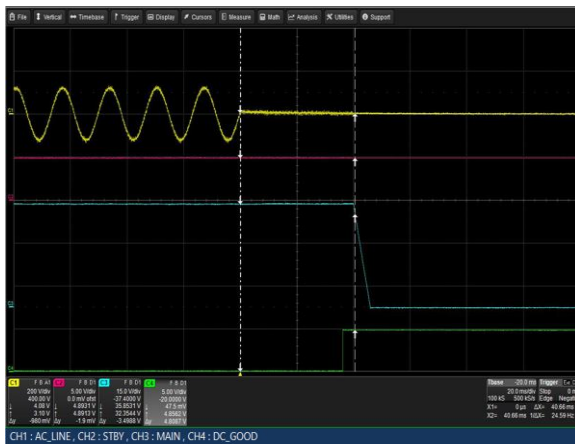
Figure 47: LCM3000U-T Hold-up Time
