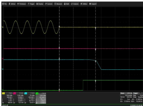
Figure 75: LCM30007-T Hold-up Time
