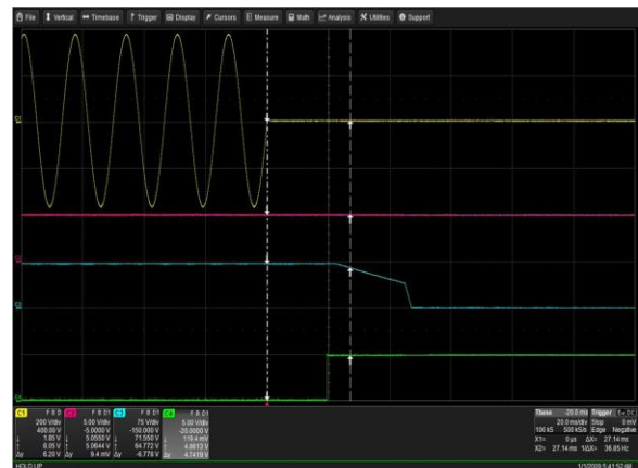
Figure 76: LCM30007-T Hold-up Time
