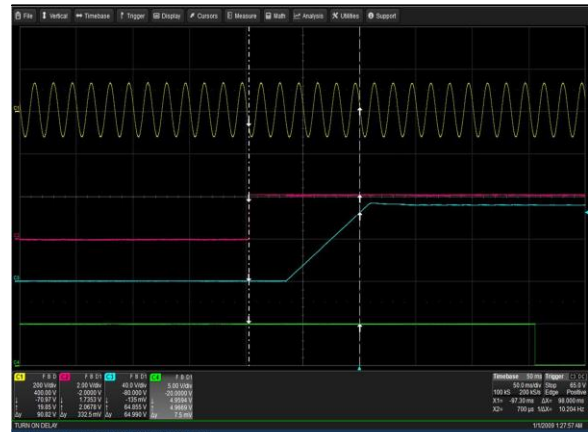
Figure 72: LCM30007-T Turn-on delay via INH_EN
