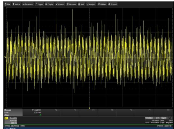
Figure 84: LCM30007-T Ripple and Noise Measurement Vin = 230VAC Load: I_o = 41.7A (72V), I_{sb} = 2A Ch 1: Vo
