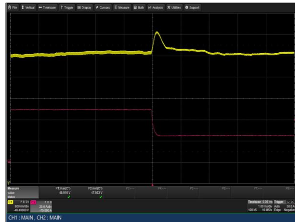
Figure 66: LCM3000W-T Transient Response - V_o Deviation 100% to 50% load change 1A/uS slew rate V_{in} = 230VAC Ch 1: V_o Ch 2: I_o
