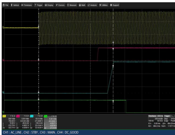
Figure 45: LCM3000U-T Turn-on delay via AC mains
