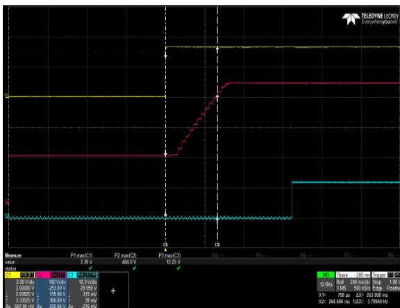
Figure 3: AIF06ZPFC-01L Turn-on delay via PF ENABLE Vin = 115VAC Load: Io = 0A Co = 2000uF Ch 1: PF ENABLE Ch 2: Vo Ch 3: LD ENABLE
